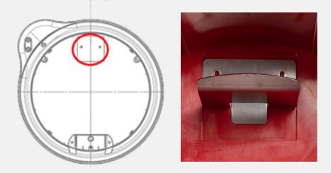
Step 3: By loosening and tightening the hexagon cap screws the bracket can moved up and down. You can use this to adjust the hanging bracket to the desired height.
