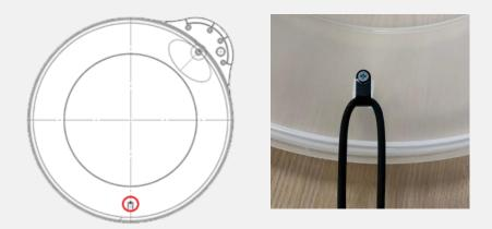
Step 5: Keep the lid of the cup and plug the adapter into a wall socket to start powering the Cabinaid Pro. If all steps were followed correctly the Cabinaid should give an Audible alarm and the LED lighting should be flashing.
