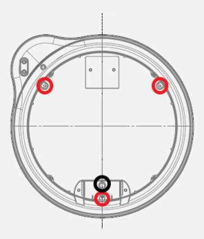
Step 4: After marking the holes put the Cabinaid storage compartment aside and use a drill to make the holes in the wall.
